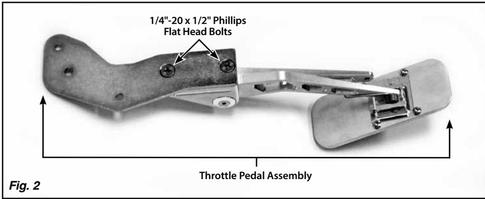
**Step 5:** Position the upper and lower pedal arms in the pedal cradle. Install the pedal axle through the left side of the pedal cradle, through the splined bushing, and out the right side of the pedal cradle. Reinstall the #10-32 x 3/8" flat head screw and aluminum end washer onto the end of the pedal axle and tighten. Check the Throttle Pedal and make sure that it is not binding.
