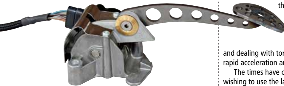
The Lokar ETC with the Lakester pedal assembly in position. Once mounted in the car you can adjust pedal pad to final adjustment to suit your foot position needs.
