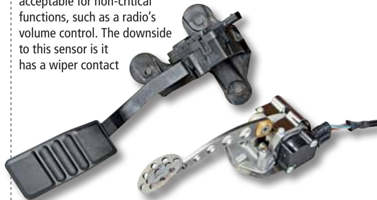
At the top is a typical Ford (Mustang) electronic throttle control (drive-by-wire) with the Lokar Performance ETC (with Hall-effect sensor) with a Lakester-series pedal assembly attached.
