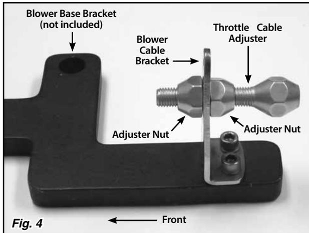
**Step 6:** Remove the front adjuster nut from the throttle cable adjuster, and insert the throttle cable adjuster into the blower cable bracket. Position the rear adjuster nut so that the blower cable bracket is approximately centered on the threaded part of the throttle cable adjuster. (**NOTE:** If a Lokar Kickdown Cable is also being installed, you will need to install the kickdown mounting bracket onto the throttle cable adjuster at this time.) Reinstall the front adjuster nut. **Fig. 4**
