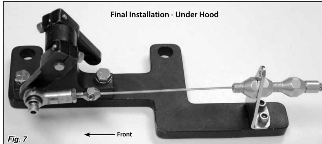
**NOTE:** Once the Throttle Cable is installed, make sure that the Throttle Pedal is completely floored when the throttle is wide open. If the Throttle Pedal is not completely floored at wide open throttle, you will need to either adjust the pedal itself or install a pedal stop.
