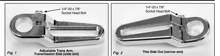
Transmission *Note:* Original trans arm may look different or be positioned differently. If the original trans arm is welded to the selector shaft 1/4"-20 x 7/8" and it interferes with the new adjustable Socket Head trans arm, it will need to be removed using Bolt a cutoff wheel. 5/16" Bolt with Trans Selector Shaft 1/2" Hex Head (not included) (not included) Adjustable Trans Arm Fig. 3 To Shift Linkage
