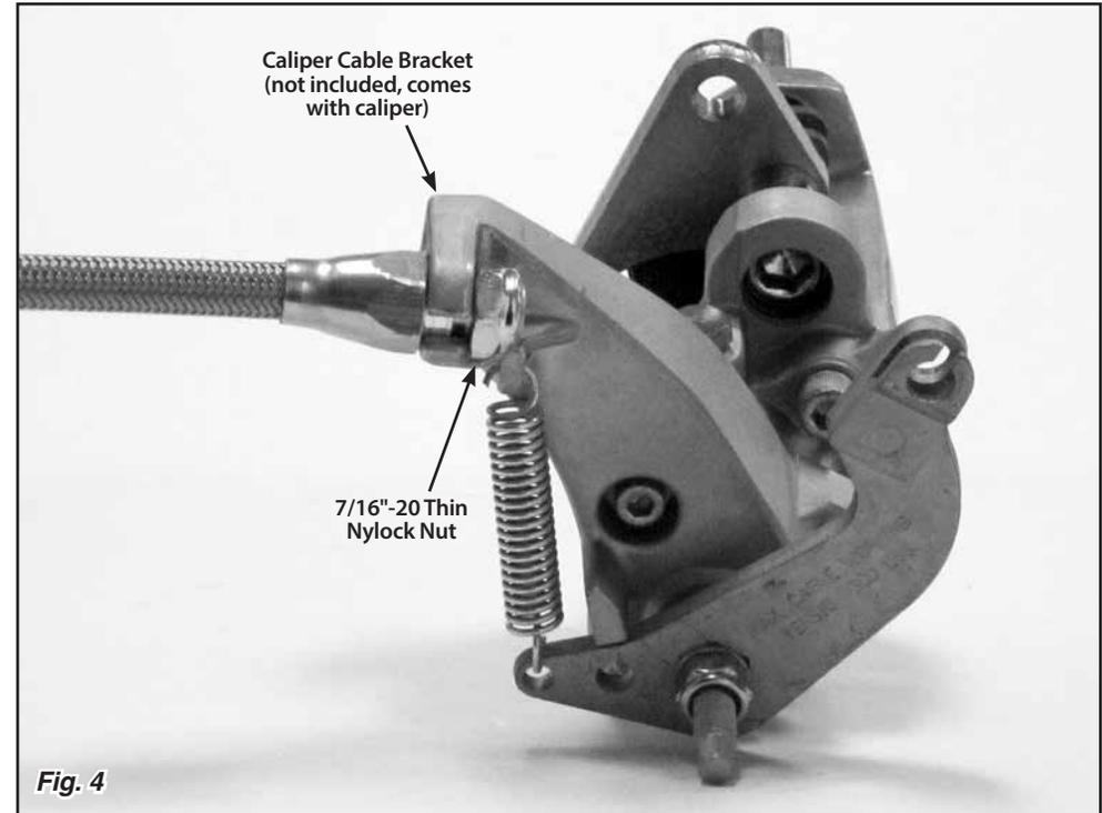
**Step 4:** Route the cable housings up to the cable adjuster bracket. Be sure to keep the cable housings a safe distance away from the exhaust and from any moving parts. Cable housings that are damaged or melted will not be covered under warranty.
