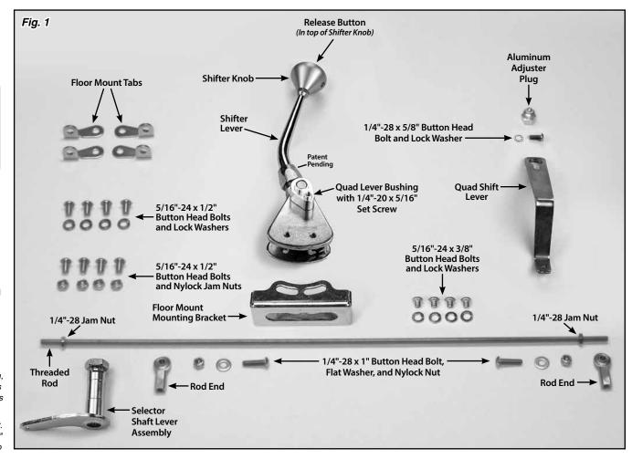
To shift from Park directly to Drive, depress the release button and hold it down while moving the shifter lever, and the shifter lever will stop in the Drive position. Once you release the button, the shifter lever will allow you to move into the next lower gear. You must depress the button to shift down again.
