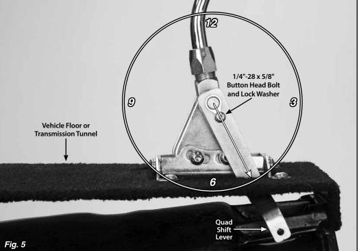
Step 5: There are two pairs of floor mount tabs in the Shifter Kit. Which pair goes where will depend on if you are mounting the Shifter above or below the floor. See Fig. 3 to determine how the floor mount tabs need to be positioned for your particular application.
