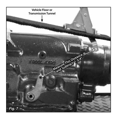
Step 12: The threaded rod will connect the quad shift lever to the selector shaft lever. Check to make sure that nothing will interfere with the travel of the threaded rod.
